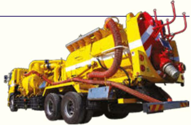
“swell,” owned by REVACS Corporation, is an ultra-high strength vacuum truck with an air flow of 140 m<sup>3</sup>/minute, one of the highest in Japan. There are only three of these unique trucks in Japan. This service, specialized in environmental infrastructure cleaning at plants, offers the cleansing of tubs, plumbing, tanks and other parts of plant waste water treatment facilities, at low costs and rapid speeds with this highly functional truck that other companies do not possess.
